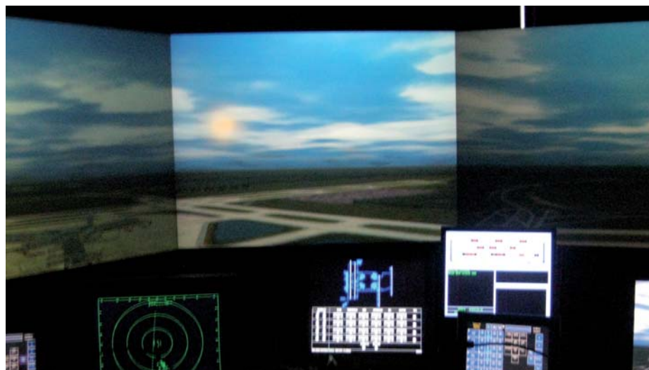
ATC tower simulator at Middle Georgia Aviation Campus. The voice recognition system is even able to interpret accented English first time and pass on instructions to AI traffic.
