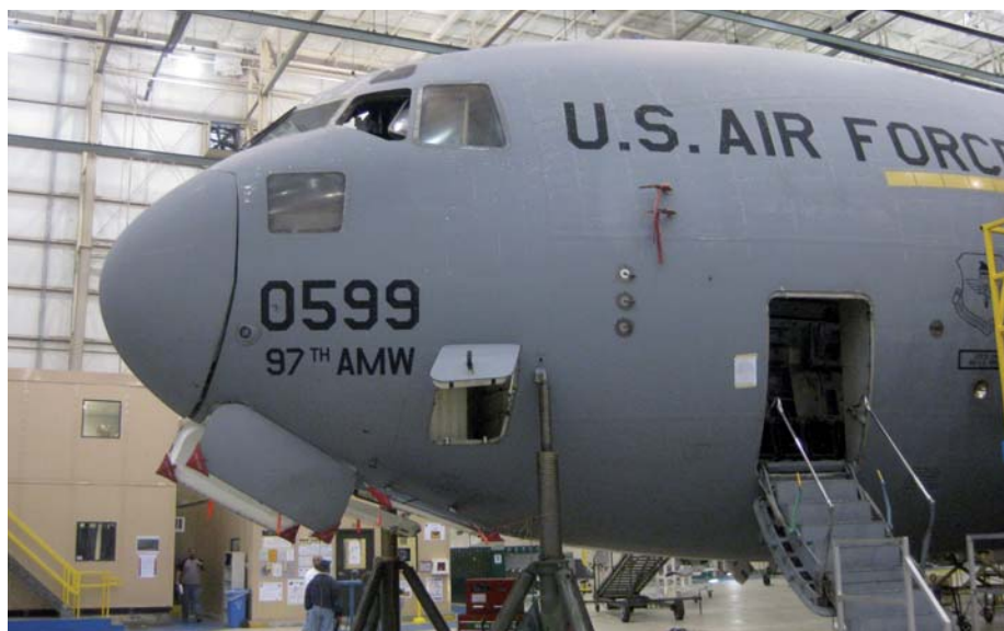
Boeing C-17 at Warner-Robins AFB. Note the sandblasted paint — a sign of some hard usage.
